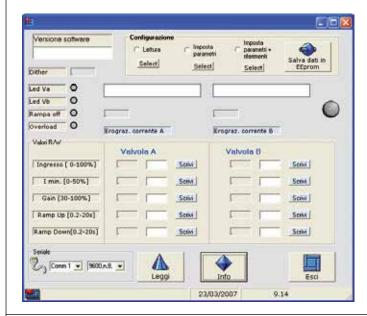
DG program for the digital adjustment of the parameters of the REMS and REMD boards.
