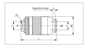
Flow control valve using non compensated throttling.
