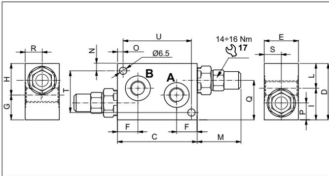
The direct acting compensator valves with CMP04 type cartridge protects the hydraulic components from impact or peaks in pressure. It raises the safety level by making it impossible for the plant operators to set a higher pressure rating, than that specified in the catalogue. It has a pack spring with a mechanical stop (only standard screw and nut). The body is in high-resistance aluminium and the cartridge is in galvanised steel.
