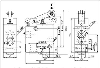
Fixing screws UNI 5931 M8x50, material specifications 12.9 Tightening torque 8 Nm / 0.8 Kgm
