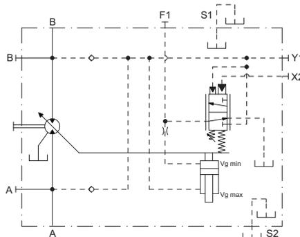
The hydraulic limiting device makes possible to reduce the pressure setting of ROE control by means of an external pilot pressure applied at port X2. The ROE control pressure setting is reduced proportionally to the pilot pressure in the ratio of 1/17 (for each pilot pressure bar, the preset operating pressure is reduced of 17 bar) [170 psi each 10 psi of pilot pressure]. Max permissible pilot pressure at port X2 = 100 bar [1450 psi].
