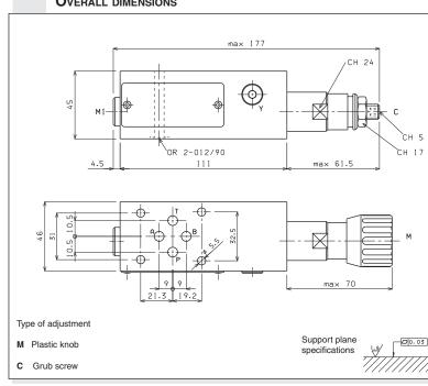
1 = max. 60 bar (white spring) 2 = max. 120 bar (yellow spring)
