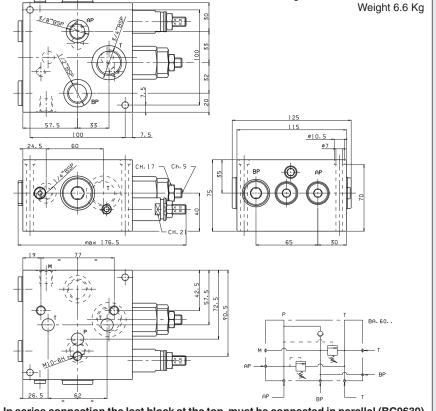
In series connection the last block at the top, must be connected in parallel (BC0630) only for mounting CETOP3/NG06 modular valves.
