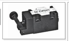
Max. pressure ports P/A/B 320 bar Max. pressure port T 160 bar 60 l/min Max. flow Minimum operating force - see note (\*) 2,5 Kg Maximum operating force - see note (\*\*) 13 Kg Cam angle 27° Fluid viscosity  $10 \div 500 \text{ mm}^2/\text{s}$ Fluid temperature  $-25^{\circ}\text{C} \div 75^{\circ}\text{C}$ Ambient temperature -25°C ÷ 60°C class 10 in accordance Max. contamination level with NAS 1638 with filter  $\beta_{25}\!\!\geq\!\!75$
