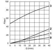
**0** = VMP10.0.. - **1** = VMP10.1.. - **2** = VMP10.2.. - **3** = VMP10.3.. Fluid used: mineral based oil with viscosity 46 mm<sup>2</sup>/s at 40°C.
