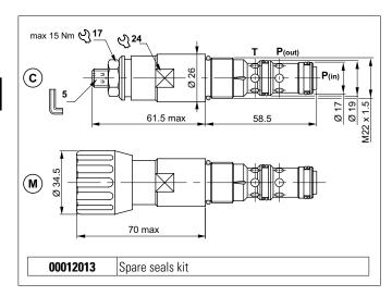
The pilot-operated sequence valve feeds a secondary branch of a circuit when a set pressure value is reached, guaranteeing minimum variation of the set pressure with flow alterations of up to 90 l/min. Slight leakage is tolerated for this type of valve.
