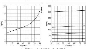
**1** = CVS20.1.. - **2** = CVS20.2.. - **3** = CVS20.3.. Fluid used: mineral based oil with viscosity 46 mm<sup>2</sup>/s at 40°C.
