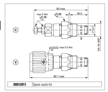
The direct acting sequence valve feeds a secondary branch of a circuit when a set pressure value is reached and suppresses the primary pressure.
