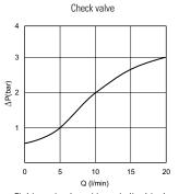
Fluid used: mineral based oil with viscosity 32 mm²/s at 50°C.
