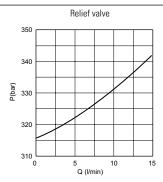
Fluid used: mineral based oil with viscosity 32 mm<sup>2</sup>/s at 50°C.
