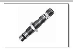
The inductive proximity sensors make it possible to detect metal objects; the operating principle is based on a high frequency oscillator which produces an electromagnetic field in the immediate vicinity of the sensor.
