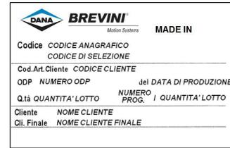
HPU are identified by a part number and an ordering code on the documents provided with the units (invoice). All requests for explanations or replacement parts must be accompanied by the identification codes described above.
