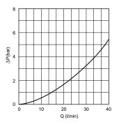
Fluid used: mineral based oil with viscosity 15 mm<sup>2</sup>/s at 40°C.
