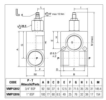
The pilot-operated relief valve limits the pressure in the hydraulic circuit. Slight leakage is tolerated for this type of valve.
