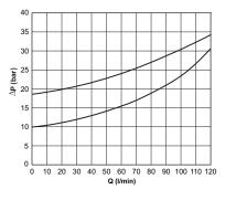
Pressure drops with compensator setting at 10 and 19 bar
