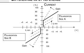
For being able to command a proportional valve double solenoid with a differential input command voltage in income at contact 9 of REMD is necessary not to connect the contact 10 of REMD.
