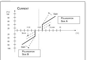
For being able to command a proportional valve double solenoid with a positive command voltage in income at contact 9 of REMD is necessary to connect the contact 10 of REMD a resistive load:
